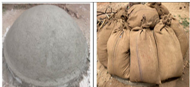
Figure 6. EPSC spherical shell a) freshly casted b) loaded with uniform pressure
